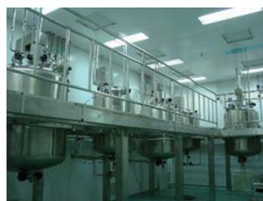
Buffer preparation system manufactured by us prepares the buffers made of multiple liquids and mixes them in the buffer preparation tanks for use in diafiltration processes.
