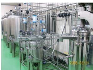
Medium preparation system manufactured by us, which consists of tanks, pumps, heat exchangers, filters, valves, piping and instruments, is used to facilitate the growth of biological materials such as mammalian, yeast, insect, or bacterial cells.
