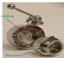
Split butterfly valves sourced from suppliers can transfer products in an air-tight condition to avoid cross contamination and can protect the operator and the operational conditions.
