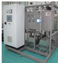
CIP/SIP units manufactured by us which are used for cleaning and sterilisation of the vessels, piping and the whole system.
