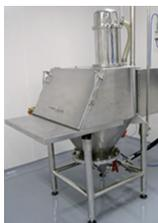
Discharging machines manufactured by us are used in discharge of active pharmaceutical ingredient from aluminum drum or bag to the bin.
