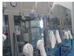
A restricted access barrier system (RABS) manufactured by us provides an enclosed environment to reduce risk of contamination.
