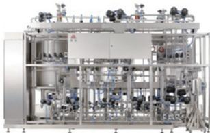
Preparation mixing vessels manufactured by us which are used for mixing raw materials with water, which may involve multiple tanks for preparing liquid solution for injectable pharmaceutical products and oral liquid pharmaceutical products.
