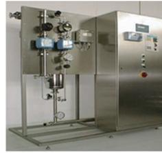
Purified water distribution skids manufactured by us which are used to facilitate the control and monitoring compliance using modular design and plug-and-play concept
